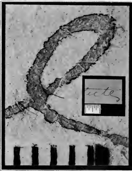
FIG. 146—A nigrisine ink line with microscopic black edges. Actual size and enlarged x 21.
